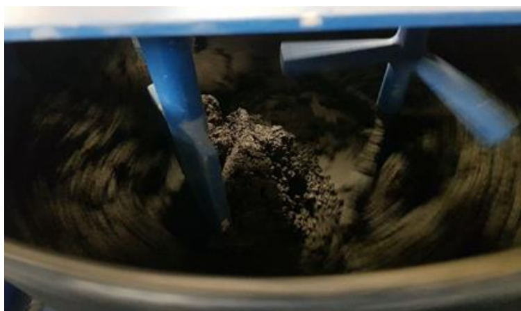
Figure 9. Sample preparation with electric mixer
