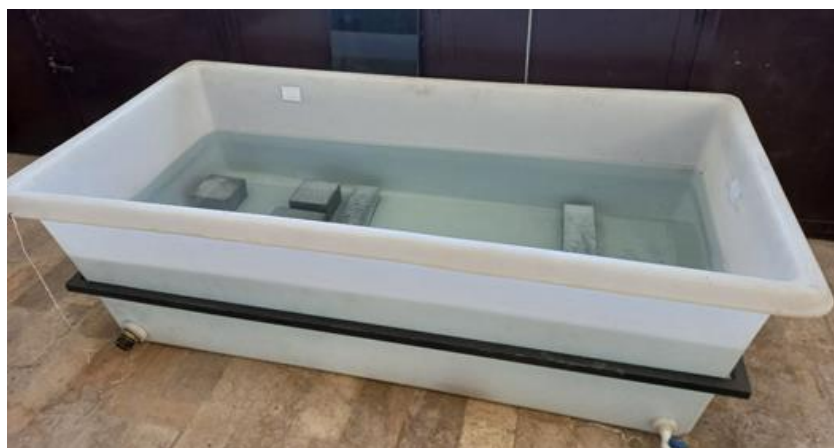
Figure 8. Concrete curing water bath
